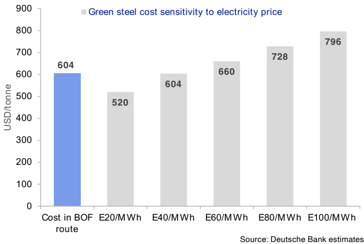
Figure 1: BOF route vs green steel cost sensitivity to electricity costs (iron ore, coal at DB's long-term estimates, CO 2 = E80/t)
